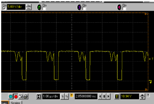
FIGURE 7. BOOST SWITCH NODE AT 100mA (PARTIAL DISCONTINUOUS)
